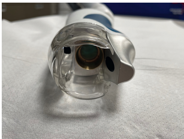
Figure 1. The hand piece of the integrated device is equipped with cold air cooling combined with a built-in smoke evacuator.
